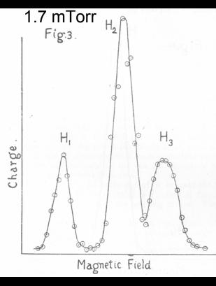
→ H<sub>3</sub><sup>+</sup> formed in secondary reaction
