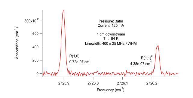
Finally, the expansion was probed at different axial positions downstream of the nozzle. Observed linewidths decreased by a factor of 25% when moving from 1 to 1.5 cm.
