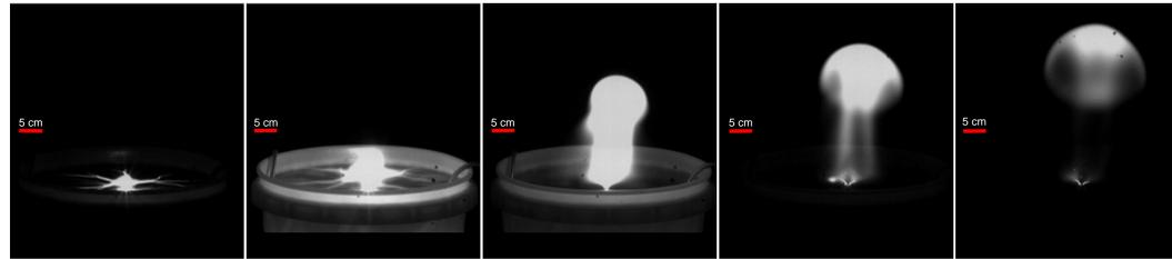
Figure 4. A series of images obtained from one plasmoid discharge at 7000 V. Images recorded with a Phantom V5.2 high-speed camera at 1000 fps (990 μs exposure time) at a resolution of 1152 x 896 pixels (images are cropped to remove dark space). Scale bar included is 5 cm.
