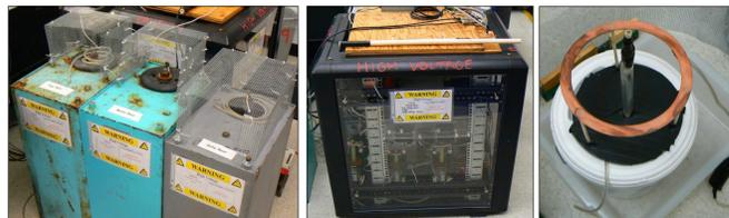
Figure 2. Photos of (left to right) capacitor bank, switching box, and electrode setup.
