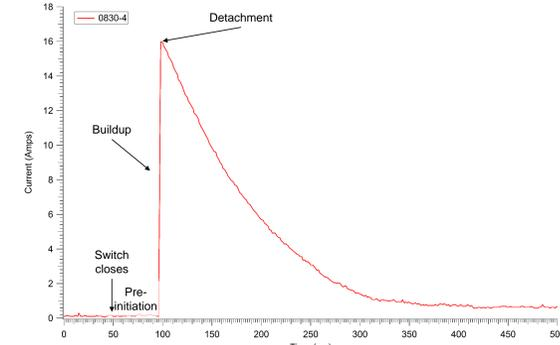
Figure 3. A current trace of a typical ball plasmoid discharge. Phases of the discharge are labeled.
