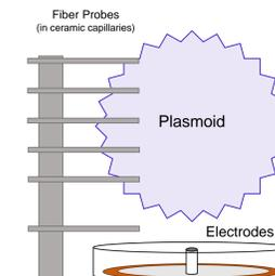
Figure 5. Schematic of probe spectroscopy setup. Probes will be oriented vertically along the discharge axis.
