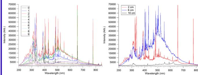
Figure 4. Example preliminary emission spectra collected from plasmoid discharges. Left: series of spectra collected from one discharge, right: series of spectra collected at different heights relative to cathode level.
