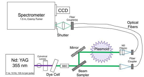
Figure 6. Proposed broadband dye laser configuration for absorption spectroscopy measurements.
