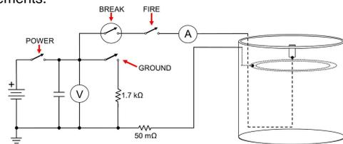
Figure 1. Schematic of discharge circuit. A and V are a Hall effect sensor and voltage divider, respectively.
