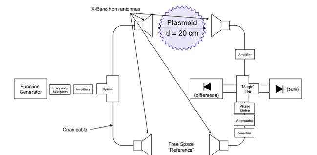
Figure 7. Proposed design of full-bridge X band microwave interferometer for electron density measurements.
