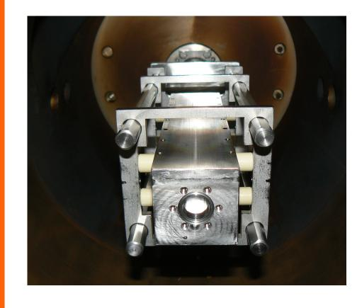
The oven was recently redesigned to hold more sample and work with samples that melt, such as PAHs. We want to work with PAHs to understand cooling of large molecules.
