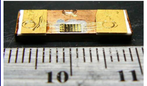
In order to perform highresolution spectroscopy at 1185 cm<sup>-1</sup> we use a quantum cascade laser (QCL) provided by collaborators at Princeton
