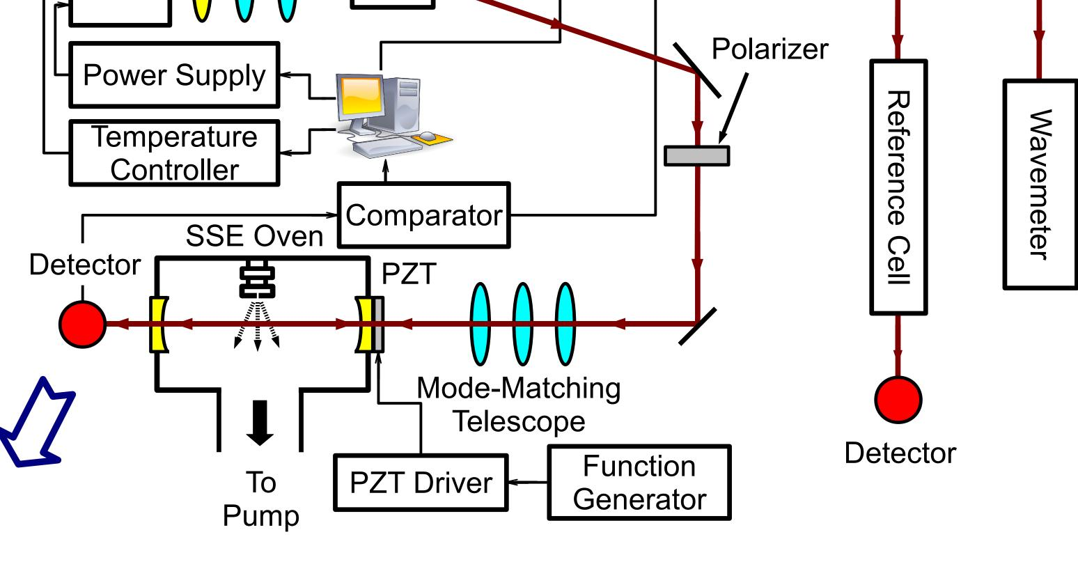
As the cavity length changes, the laser comes into resonance with the cavity, leading to a buildup of signal on the detector. When the signal reaches a predefined threshold, the AOM is turned off, and the decay of light from the cavity is measured. We place a high temperature supersonic expansion source inside the cavity to generate cold gas phase C<sub>60</sub> and use our spectrometer to measure the vibrational absorption spectrum.
