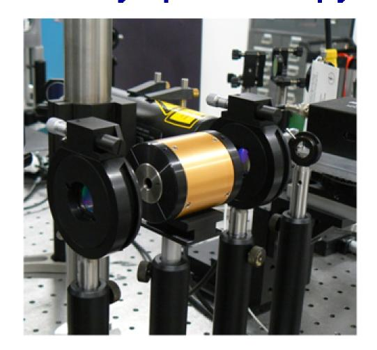
➤To eliminate feedback from our high reflectivity mirrors in the experiment we are working with Optics For Research (OFR) developing an optical isolator at ~8.5μm
