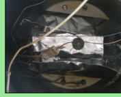
> 600 °C oven and supersonic expansion for rotationally cold gas phase C 60
