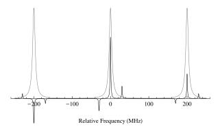
**Fig. 7.2** The spectrum of a laser modulated for use in a NICE-OHMS setup overlaid with three optical cavity modes. Note the two sets of sidebands on the laser, in this example spaced at 30 MHz for cavity locking and 200 MHz for heterodyne detection. The second set of sidebands must be spaced at an integer multiple of the cavity FSR. They are most commonly spaced at a single FSR, but can be spaced at two [5] or even nine [6] or more times the free spectral range
