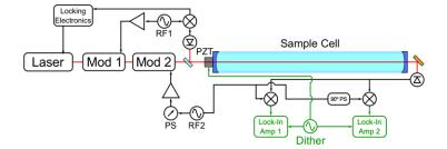
**Fig. 7.1** A generic NICE-OHMS experimental layout. The green components are utilized only in wavelength modulated (wm-NICE-OHMS) setups. For fm-NICE-OHMS, the final experimental signals are taken directly from the mixer outputs. Alternatively, in velocity modulation setups, as described in Sects. 7.3.2.2 and 7.3.2.3, the 'dither' is applied to the discharge voltage (not pictured here) across the cell, inducing an alternating Doppler shift of the ions within the cell
