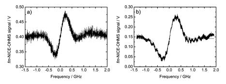
**Fig. 7.5** fm-NICE-OHMS spectra of HO<sub>2</sub> with fits from Bell et al. [5] (a)  ${}^{q}P_{1}(12)$  transition at 6623.32 cm<sup>-1</sup>, (b)  ${}^{q}P_{2}(10)$  transition at 6623.57 cm<sup>-1</sup>
