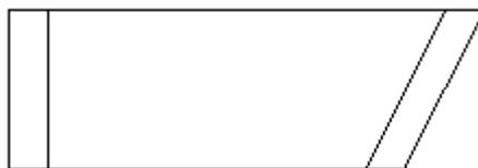
Figure 2.2: Illustration of the crystal cell. The light is input through the left side and vertically deflected by the tilted window as the light leaves the cell. The vertical deflection is directly related to the refractive index of the *para*-hydrogen crystal.
