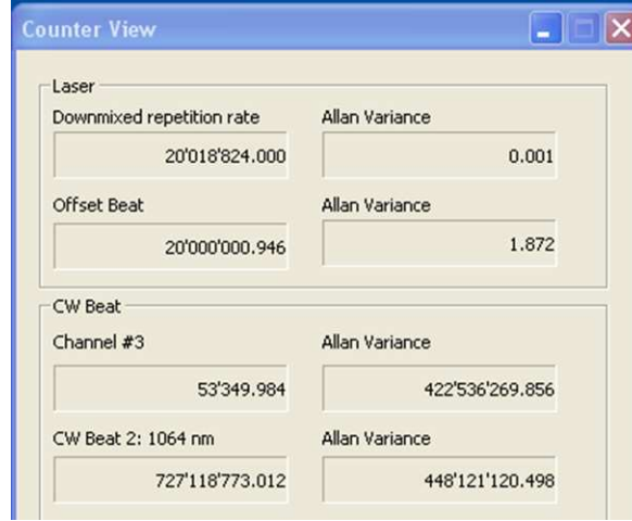
Figure 3.15: A screenshot of the “Counters View” box of the Fiber-comb software. The top value is the “Downmixed Repetition Rate” used to determine the repetition frequency of the fiber-laser as described by Equation 3.6 in Section 3.3 and as used to adjust the fiber-laser’s repetition frequency lock. The second value is the absolute value of “Offset Beat”, used as part of Equation 3.4 to determine the unknown cw laser’s frequency. “Channel #3” is the counter reading from the visible channel which is used to measure the absolute value of the beat frequency of the Ti:Sapphire laser. “CW Beat 2: 1064 nm” is the counter reading from the IR channel which is used to measure the absolute value of the beat frequency of the YAG laser. The reported Allan variances (Hz) are for the last 100-1000 data points taken and are only useful if the laser is actively stabilized to something ( f_{REP} and f_{CEO} are actively stabilized, and their variance therefore has meaning).
