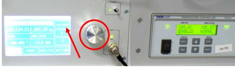
Figure 3.9: Direct digital synthesizer (DDS) on the left and the Thorlabs TC200 which controls the temperature of the periodically poled lithium niobate crystal for doubling the comb radiation.
