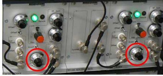
Figure 3.13: A picture of the lockboxes used for locking the carrier envelope offset (left) and frequency (right) of the fs-comb laser. The knob for adjusting the offset is circled in red. The button for turning the lock on and off glows green when engaged. The red LED to the right of the green switch is illuminated when the locking mechanism is engaged but not locked.
