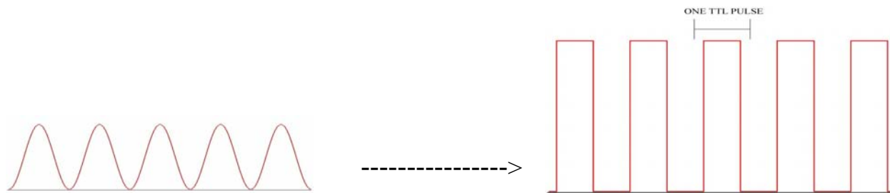
Figure 1.9: Function of TTL converters
